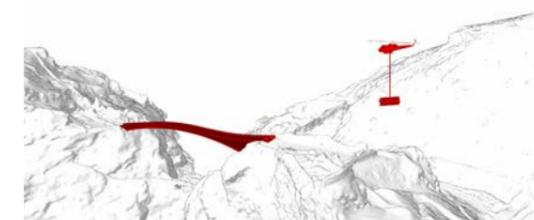
6) Removal of centring and large temporary works via cable crane
